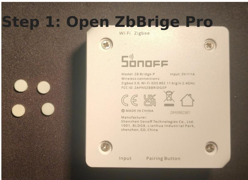
Remove the rubber feet by using e.g. a scalpel at the bottom and unscrew the 4 small phillips screws beneath.
