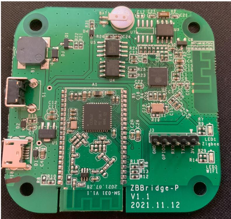
Solder 5 pins to the GND, GPIO0, RX,TX and 3V pinholes.
