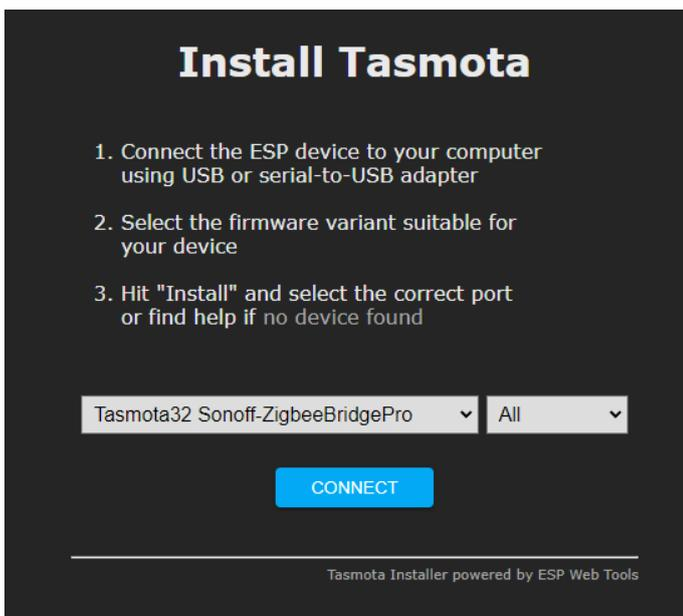
Go to the [Tasmota install website](#) and select the options **Tasmota32 Sonoff-ZigbeeBridgePro** and **All**, press connect and flash the firmware.
