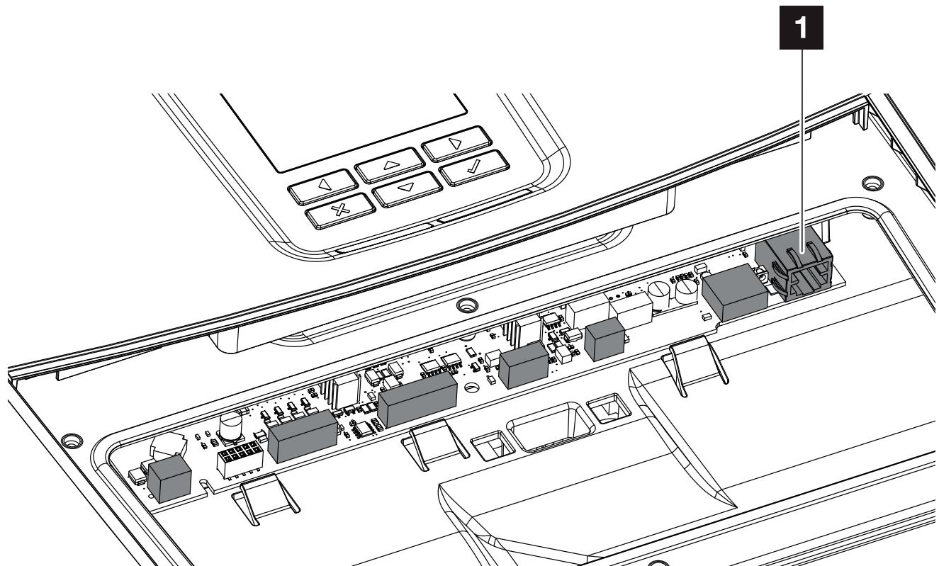
Abb. 4: Smart Communication Board - Interface
